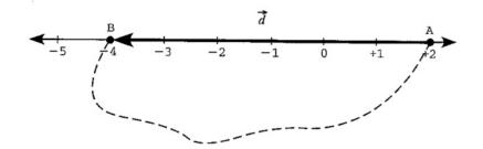
The vector drawn in bold is the displacement from point A to point B, and would be read as 6 meters to the left.
